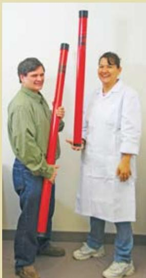
Phoenix has developed a new MT magnetic sensor, the MTC-43. The MTC-43 can replace the MTC-50 coil in many applications where lighter weight and smaller size are important factors, such as in surveys in mountainous areas.
