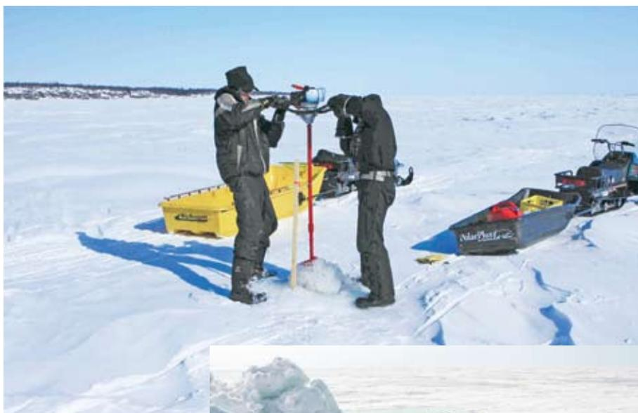
**Above:** The Canalaska survey was carried out partly offshore on the ice of Lake Athabasca. Here the crew augers through ice one metre thick before lowering electrodes to the lake bottom.
