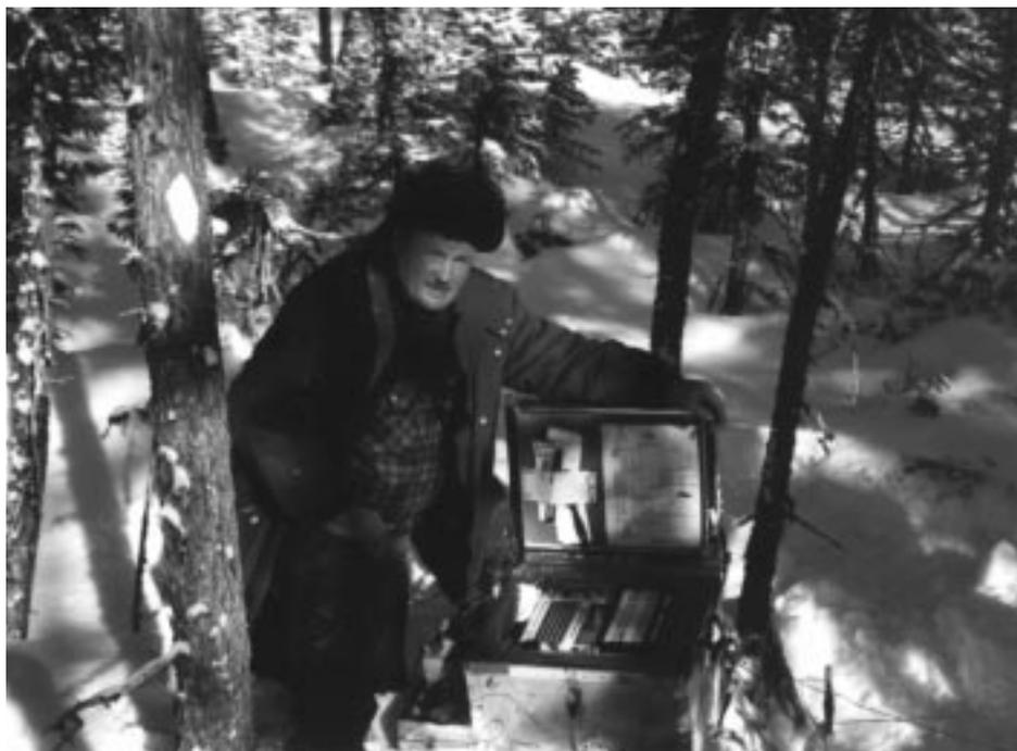
**Exciting nickel discovery: Remy Belanger (above) with his trusty Phoenix V5 IP Receiver used at the Nuinsco Mines nickel discovery near Lac Rocher, about 120 km northeast of Matagami, Quebec. A drill hole spotted on a V5 receiver IP anomaly intersected excellent thicknesses and values of nickel ore (see the Feb 1, 1999 issue of The Northern Miner). The Phase IP technique implemented in the V5 Receiver is fast in the field and excellent at locating subtle IP anomalies.**
